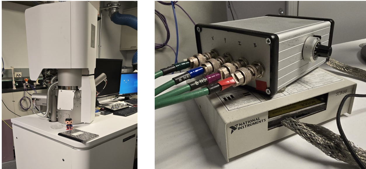
Figure 3.2: Images of the new Tescan SEM for EBL. Left: Tescan Mira 4 SEM Right: Interface buffer for EBL writing.
